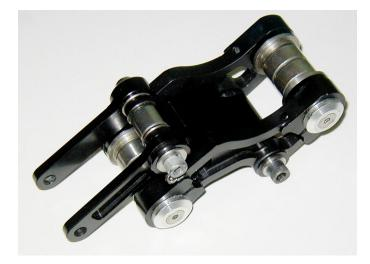
The linkage kits are CNC machined hard coat anodized aluminum. Each pivot has two Torrington full complement needle roller bearings with hardened steel bushings and are sealed with o-ring dust caps for maintenance free operation. The linkage leverage ratio has been modified for the increased travel and smoother transition through the stroke. Dust sealed thrust bushings have been added to each main pivot to keep the linkage tight and fricton free.
