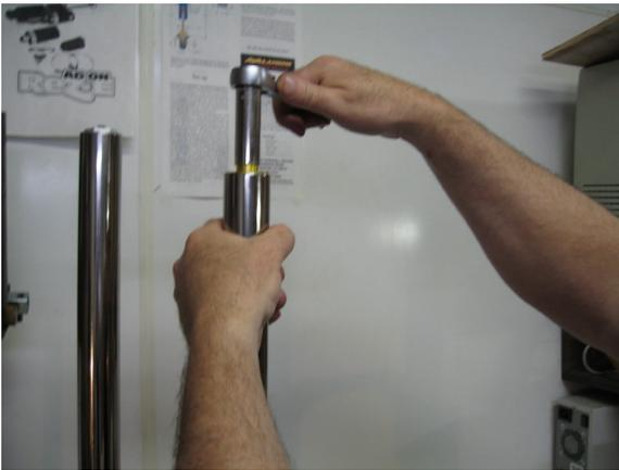
Fully extend the stanchion and cartridge rod before screwing the fork cap on. The cap does not need to be torqued, snug is sufficient as the upper crown will pinch it securely when installed.
