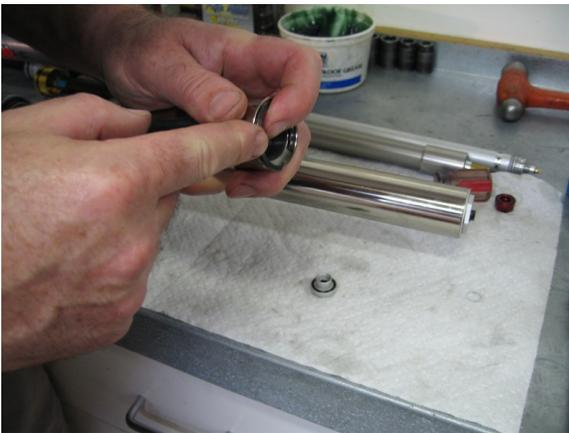
Install the snap ring provided into the groove, make sure it is fully seated.
