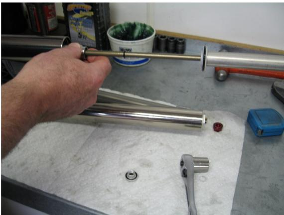
Pull the damper and spring assembly from the upper slider tube, it will take a good deal of pulling to overcome the o-ring friction to remove it
