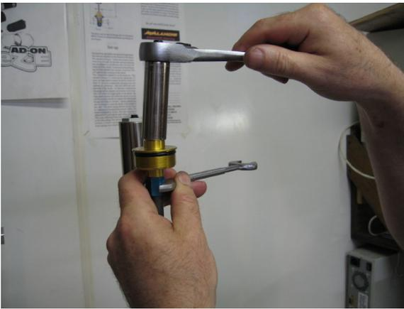
Install fork cap, be sure that the cap bottoms on rod and bring the blue jam nut up to the cap and tighten them together, approximately 1-2 foot-lbs, be careful not to over tighten as the parts will fail if over torqued.
