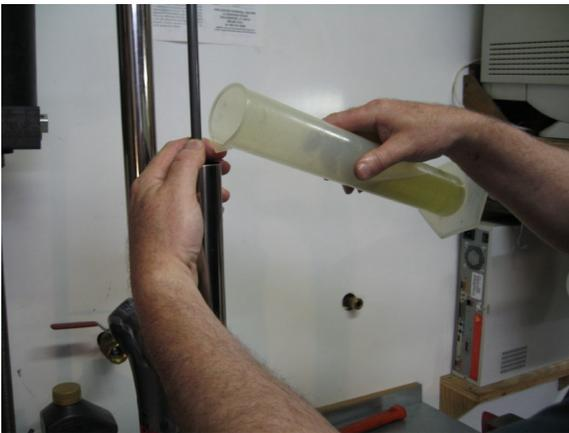
Pour approximately 300 ml of cartridge fork fluid into the damper leg, cycle the rod and stanchion up and down until all the air bubbles have dissipated.
