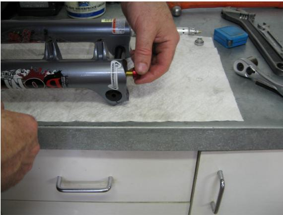
Install the o-ring and base nut.
