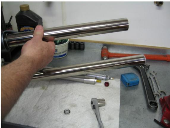
Pull the slider tube from the lower casting.
