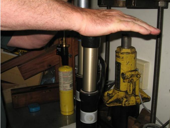
Pressurize the stanchion by placing palm of hand over stanchion and compress fork to force all air bubbles out of cartridge valving.
