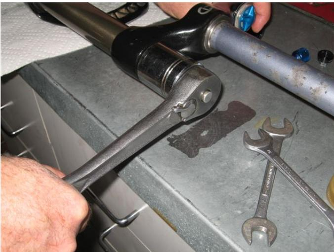
Install fork cap and tighten per Fox manual.
