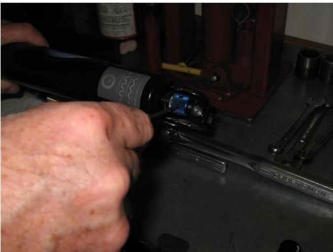
Remove high speed knob set screw and knob.
