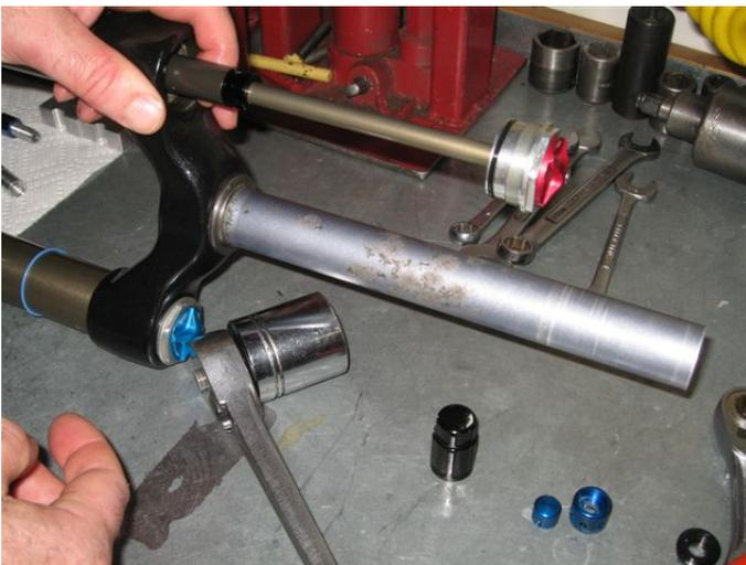
Be careful when removing, there may be excess oil that needs to be dumped. Leave the bottom-out bumper in, if needed remove it for cleaning lower casting internals.
