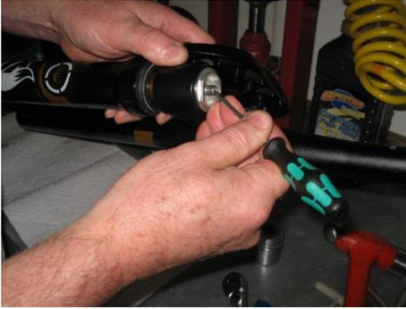
Depress the Schrader valve with a screwdriver to release the air pressure
