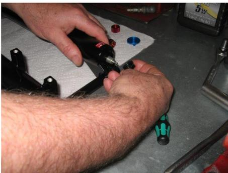
Remove the retaining nut fully
