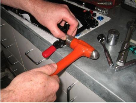
On the Sprung side tap the nut with a soft face hammer to un-seat the press fit. Push the spring assembly through the casting just like the damper side. **Do not strike the lead of any exposed external thread. It will damage it!**
