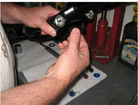
Remove the black high speed knob and expose the fork cap hex
