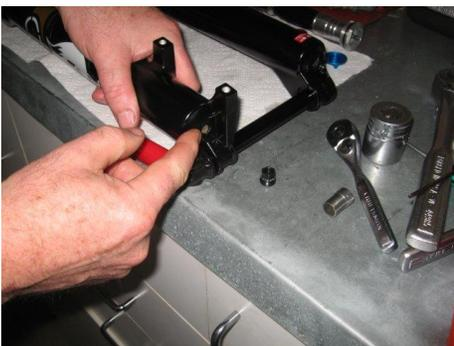
Push the sprung rod through the casting
