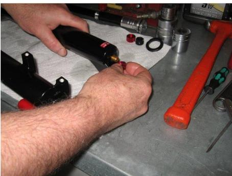
Thread the red retaining nut with included O-ring onto the assembly
