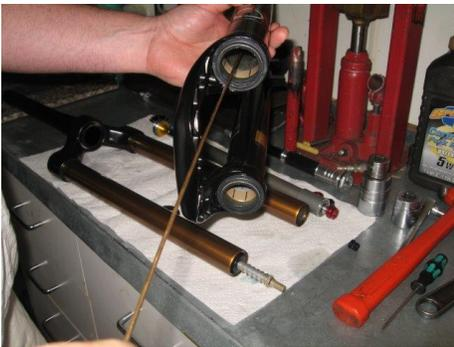
Using a bent coat hanger or welding wire create a hook and remove the factory bottom out bumper
