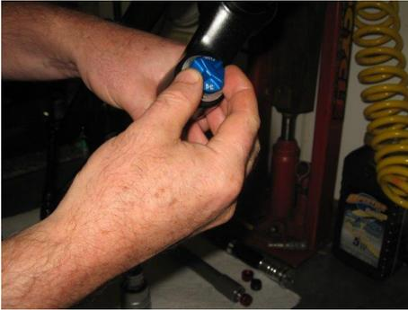
Unscrew the Air spring cap **Skip this Step if your fork has a mechanical spring**
