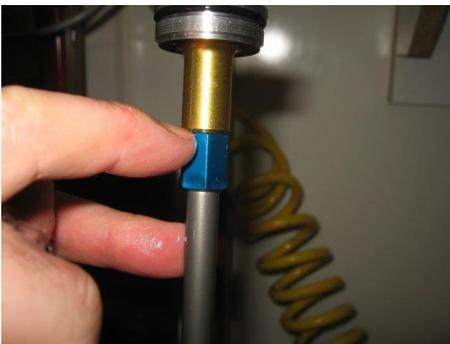
Thread the fork cap on fully to the grey shaft until the threads bottom out. **Then tighten the blue jam nut up to the gold cap.**
