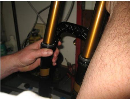
Gently reassemble the fork sliders to the lower casting. Don't force this step. It helps to get one seal started first then rock it over to the second. After both seals have accepted the sliders gently slip the tubes past the bushings.
