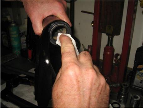
Using a clean paper towel wipe off any old grease and dirt from the dust seal
