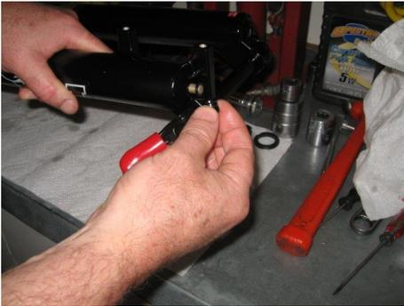
Slide the factory washer onto the air or spring shaft
