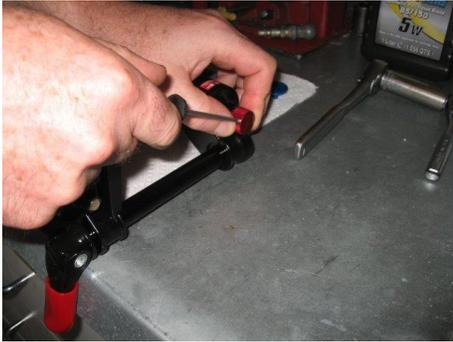
With an Allen key, remove the low speed knob.
