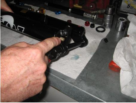
Push the assembly together and the air spring shaft should go through the casting. A small screw driver can be helpful to gently align the shaft to the hole.
