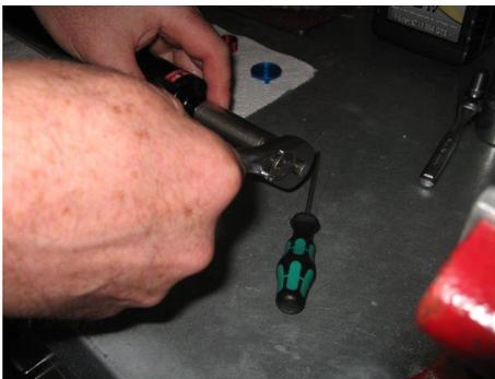
Using a 15 mm Ratchet loosen the damper retaining nut
