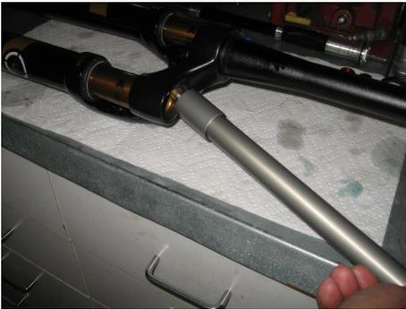
Insert the Avalanche Cartridge into the damping leg
