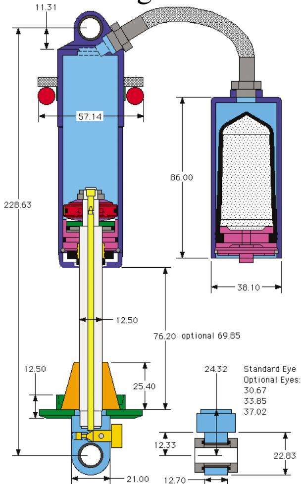
The above drawing shows the DHS-3 shock to custom installations and design of new frames.
