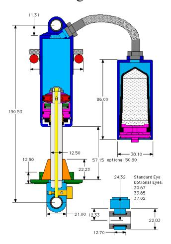
The above can be used as design info for fitting the DHS-2.25 shock to custom installations and design of new frames.
