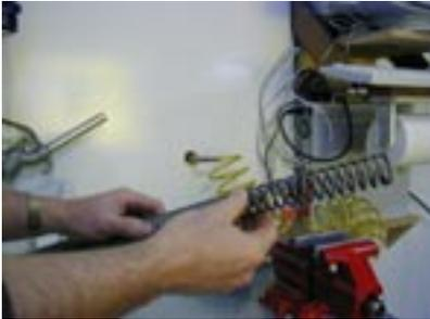
Extend cartridge rod and tilt fork at a 30 degree angle and slide fork spring over spring guide
