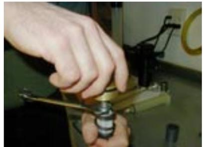
Screw on fork cap, make sure the cartridge rods bottoms on cap and bring jam nut up to contact cap
