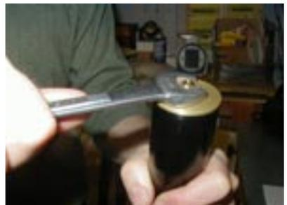
Tighten jam nut to fork cap, do not over tighten because this will damage the rod. Snug the fork cap to the upper leg hand tight.
