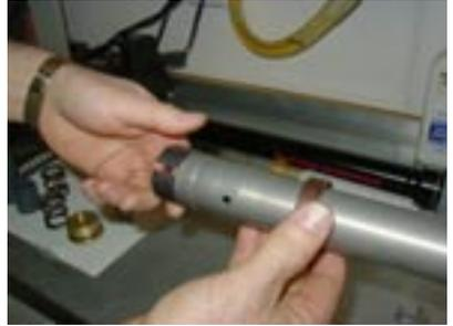
Using a 37 mm seal driver, install bushings and seal.
