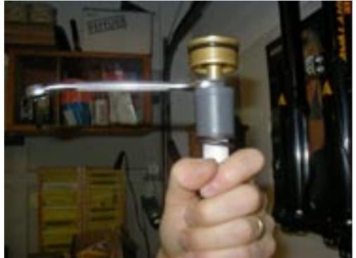
Using a 15 mm wrench loosen the fork cap from the cartridge rod by squeezing the wrenches together.
