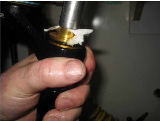
Tighten the fork cap with a 15 mm socket to 25 ft-lbs.
