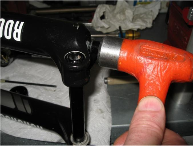
Tap the loosened bolt to relieve the lower press fit.
