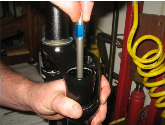
Continue filling and pumping the rod and cycling the stanchions up and down until the level stops dropping.
