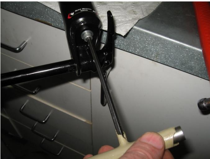
Tighten the cap screw and washer by hand snugly making sure the cartridge seats centered in the lowers. Torque to 2-3 foot-lbs.
