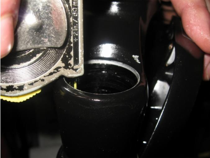
Measure from top of stanchion down to oil with the fork fully compressed and the cartridge rod pressed all the way down. The height of oil needs to be 35 for extended fork cap and 55 mm for the new flush fork cap from the top. Over fill will cause fork seal damage, under filling will cause the cartridge to suck air and have erratic damping.
