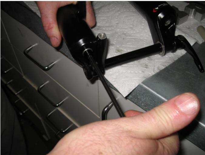
Remove the air side bottom bolt. Leave the bolt and air cap off until the damper side is set. Plug the bottom hole and fork cap with a balled up wad of paper towel to prevent dripping oil from making a mess as you install the damper.
