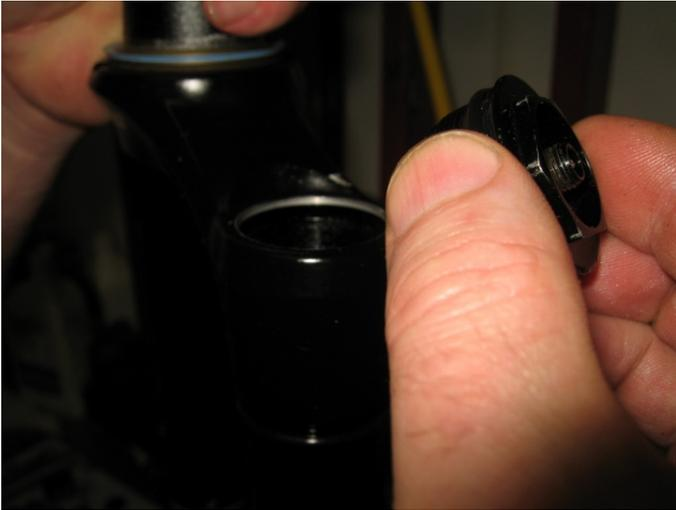
Reinstall the air side fork cap. Torque per Rockshox specs.
