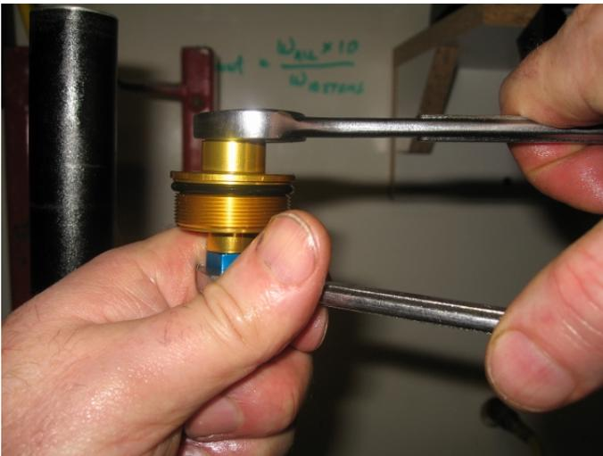
Using a  $\frac{1}{2}$  inch wrench and a 15mm, 6 point socket tighten the jam nut. **Be very careful these parts are delicate. Use a paper towel on the fork cap hex to avoid scratching the finish.**
