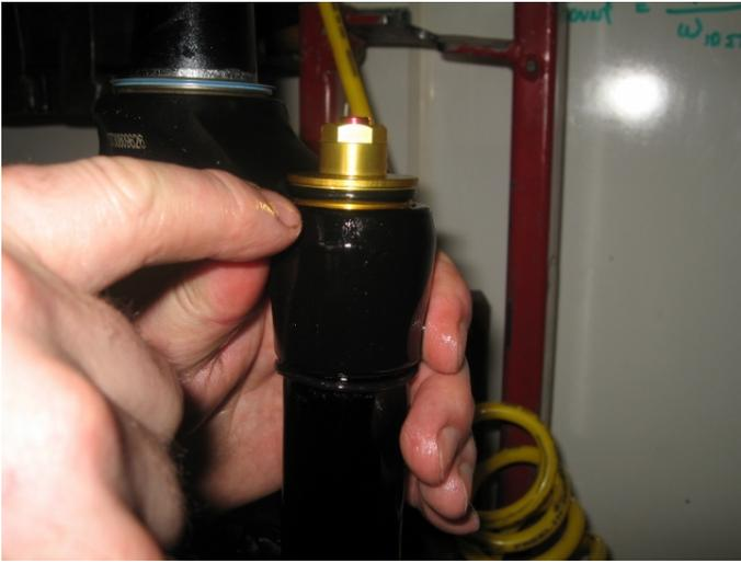
Hand thread the cap on with the fork fully extended.
