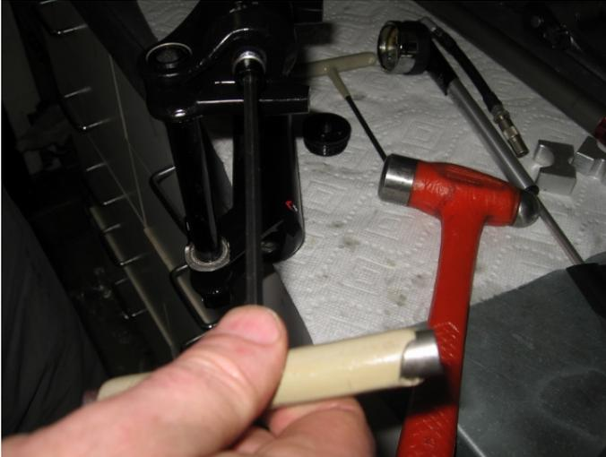
Reinstall the lower bolt, torque to Rockshox specifications. replace the gasket on bolt if necessary.
