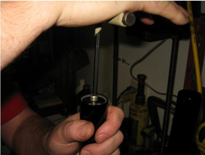
The stanchions should compress all the way down now that the pressure has been equalized. Now you are ready to add the oil, we recommend Spectro 85/150 cartridge fork fluid. Alternate oils are listed at the end of this manual, keep in mind 5 wt traditional fork oils will not work as well as the modern cartridge fork fluids.
