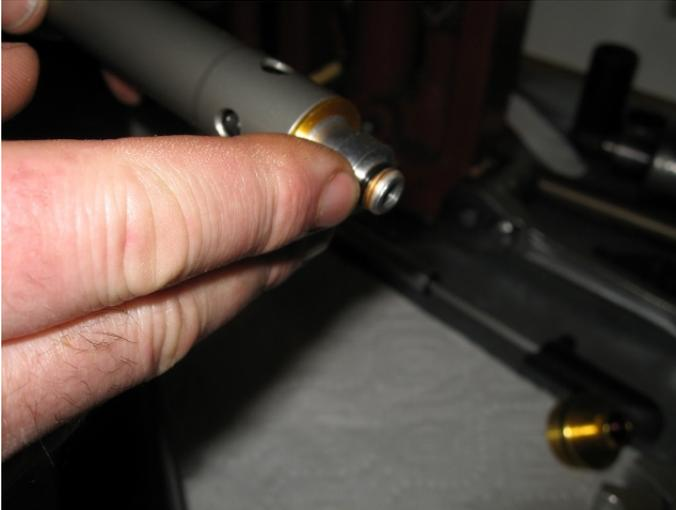
Make sure the adaptor has the 6 x 1.5 mm o-ring installed, an extra was supplied in the cartridge if damaged or needed for future reassembly.
