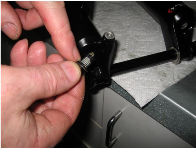
The bolt is a M8 x 1.25, one of the two methods uses a longer version of this bolt to help equalize the negative spring. You will need to purchase a 100 mm long M8 x 1.25.
