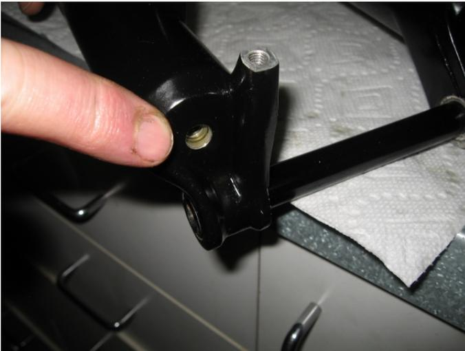
Add a small amount of air by hand to the air cap until the air shaft extend into the lowers and aligns with the hole.
