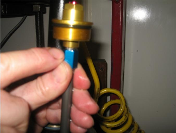
Thread the fork cap on fully to the grey shaft until the threads bottom out. **Then tighten the blue jam nut up to the gold cap.**
