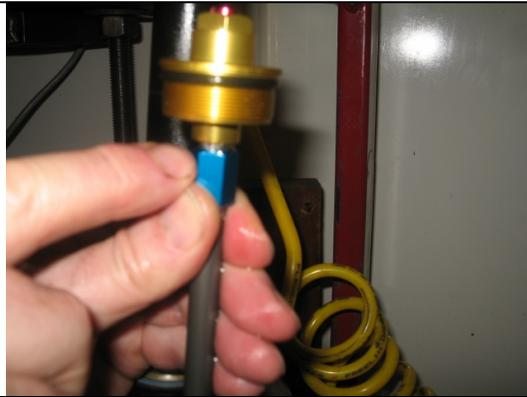
Using a ½ inch wrench and a 15mm, 6 point socket tighten the jam nut. **Be very careful these parts are delicate. Use a paper towel on the fork cap hex to avoid scratching the finish.** Tighten the fork cap with a 15 mm socket to 25 ft-lbs.
