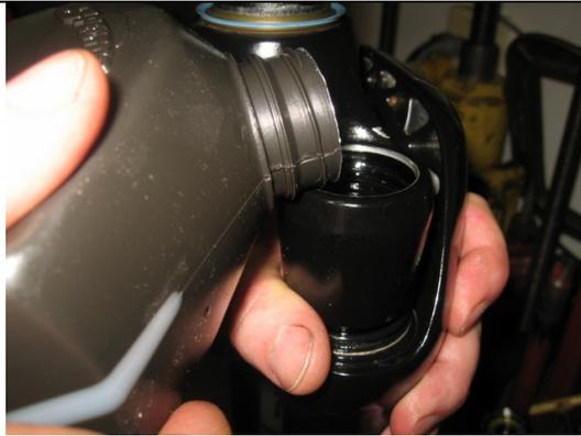
Pour in oil to fill the damper side to the top and start bleeding the air bubbles out by pulling up on the cartridge rod
