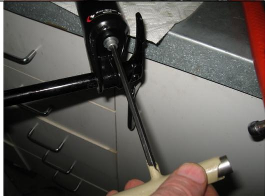
Pour in oil to fill the damper side to the top and start bleeding the air bubbles out by pulling up on the cartridge rod until the level drops, it maybe easier to temporarily attach the fork cap to create a better suction on the rod and make it easier to pull.
