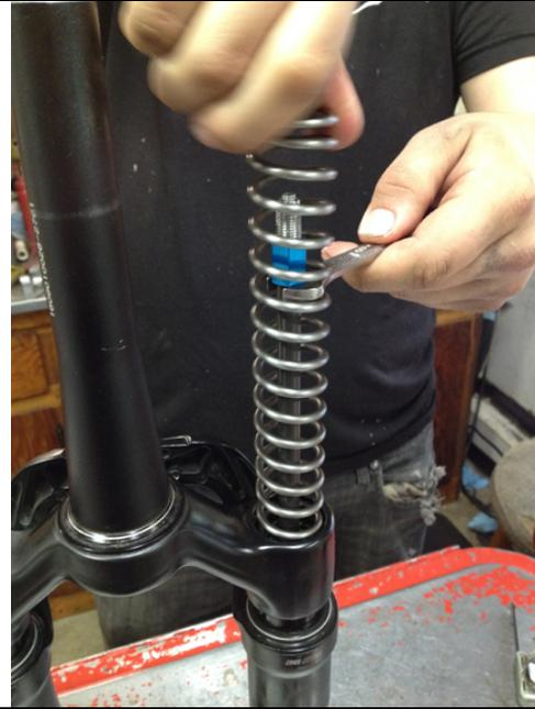
Position the 10 mm wrench under the jam nut to attach the fork cap to the rod.
