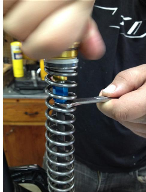
Using a ½ inch wrench and a 15mm, 6 point socket tighten the jam nut firmly hand tight (no torque requirement). **Be very careful these parts are delicate.**
