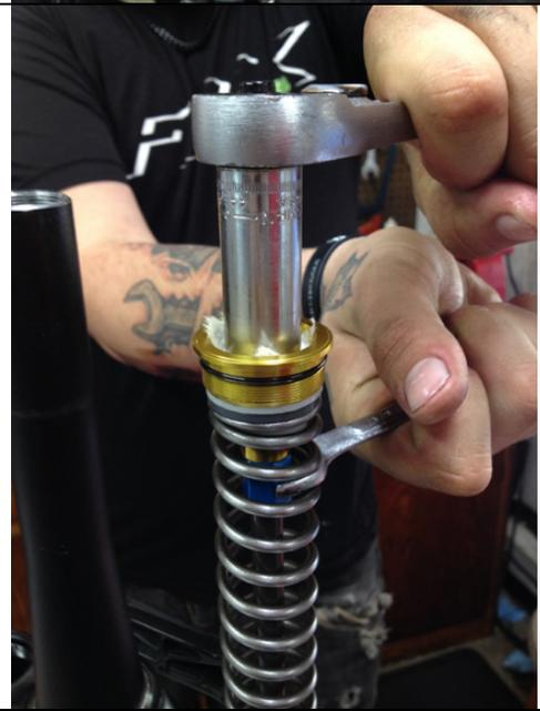
**Use a paper towel on the fork cap hex to avoid scratching the finish.** Tighten the fork cap to the stanchion with a 15 mm socket to 25 ft-lbs.
