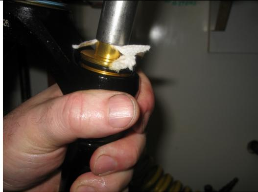
The height of oil needed for your set is specified in the setup sheet provided with your order. Over fill will cause fork seal damage, under filling will cause the cartridge to suck air and have erratic damping.
