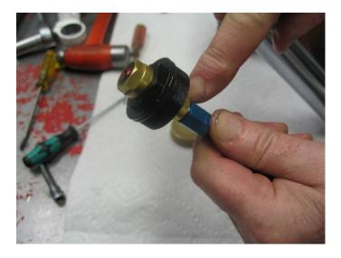
Insure the cap is screwed on all the way, there should be a gap between the blue jam nut and the gold adjuster cap.
