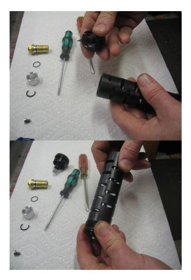
Unthread the plastic tube from the fork cap, note that this is left handed threads
