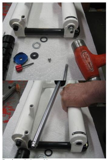
Punch out the internal insert.
