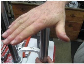
Pressurize the tube with your palm to help force the air bubbles out of the damper.
