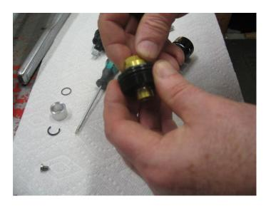
Slide the 11 mm o-ring all the way on the inside of the fork cap, this will act as a gap cushion to prevent movement under operation.
