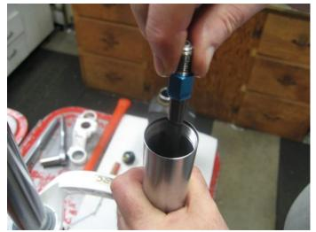
Bleed the cartridge rod and cycle the tube to remove air bubbles.
