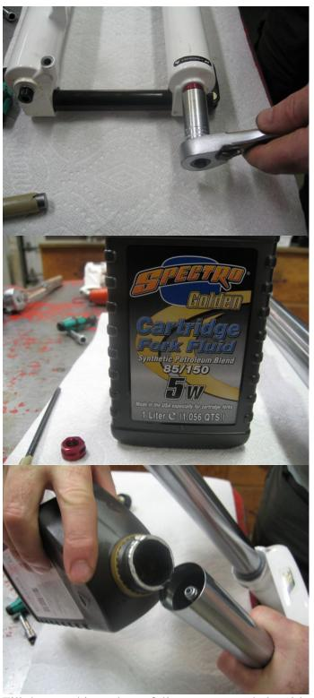
Fill the stanchion tube as full as you can to help with the bleeding of the cartridge.
