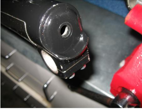
This end of the lower leg will need the internal 10 mm hole extended thru
