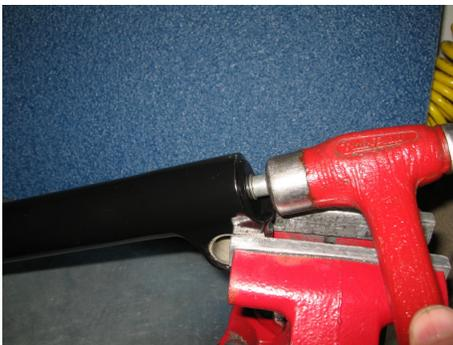
Loosen the screw more if necessary and tap until the rod is unseated
