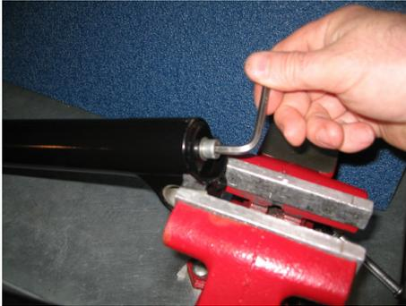
Using a 4.5 mm allen key loosen the bolt 4-5 turns
