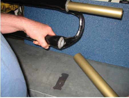
Clean the slider tube and lower leg of any remaining chips, flush if necessary
