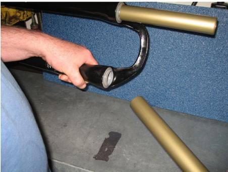
Reinsert the slider tube in the lower leg
