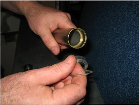
In the plastic bag provided are an oil lock ring(ABS Insert) and a snap ring
