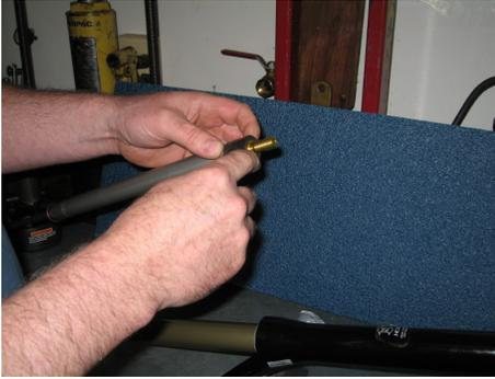
Inset the o-ring into the bottom groove
