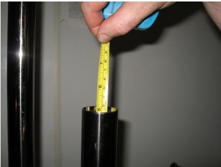
After all air bubbles are removed and damping is smooth through out the stroke. Measure down to the top of the compressed stanchion to the oil, standard is 125 mm for the Boxxer 32, and 55 mm for the Totem and the Lyrik. Using a suction tool or just dump oil out until desired height is reached
