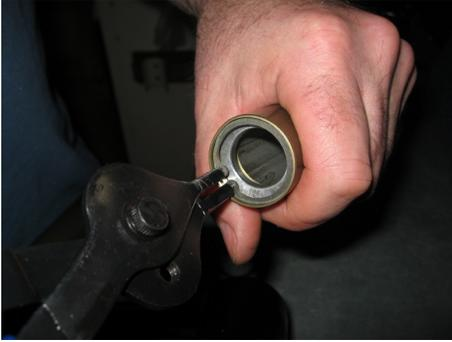
Using snap ring pliers remove the ring from the bottom of the slider leg
