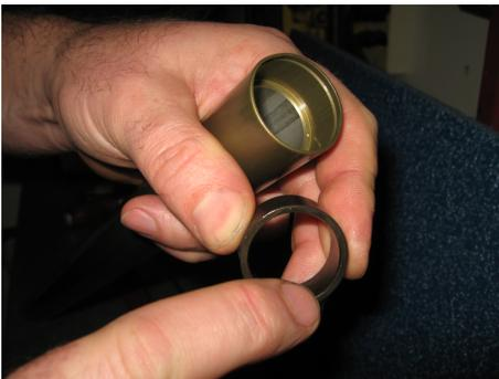
The oil lock ring will have an arrow pointing to the champher, this will face out or down to prevent damage when sliding over the ABS cone.
