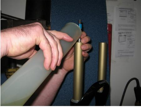
Pour oil into upper leg allowing oil to settle into the cartridge, pull the rod and stanchion tube up and down a bit until it is filled about an 100 mm from the top fully compressed
