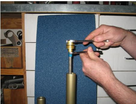
Bring the jam nut up to the fork cap and tighten with a slight squeeze on the two wrenches, approximately 10 in-lbs, be careful not to over tighten as these parts can easily be damaged
