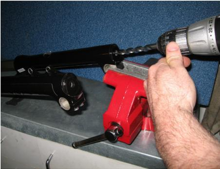
Drill with a 10 mm drill slowly blowing off the chips to avoid falling in
