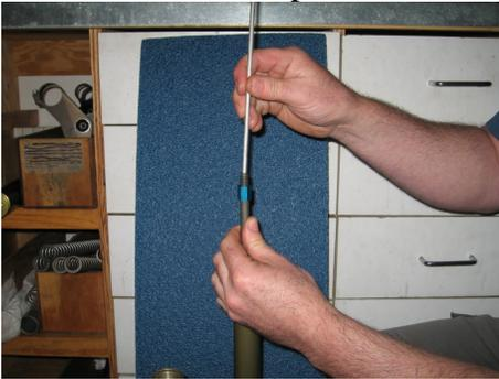
Cycle rod to remove any air bubbles and insert the rebound adjust rod. Fully compress the rod and stanchion tube.
