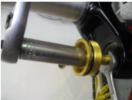
18. First Remove the Remove the Fork Cap with a ½ open
