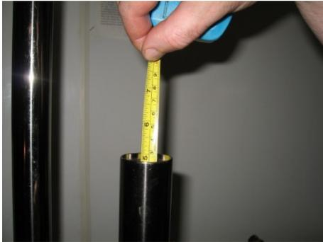
28. After all air bubbles are removed and damping is smooth through out the stroke. Measure down to the top of the compressed stanchion to the oil, standard is 55 mm for Lyrik. Using a suction tool or just dump oil out until desired height is reached
