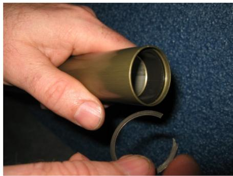
14. The oil lock ring will have an arrow pointing to the chamfer; this will face out or down to prevent damage when sliding over the ABS cone.
