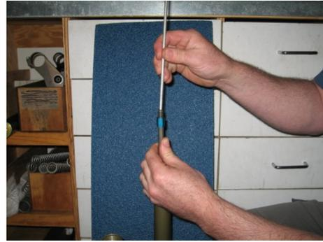
27. Cycle rod to remove any air bubbles and insert the rebound adjust rod. Fully compress the rod and stanchion tube.
