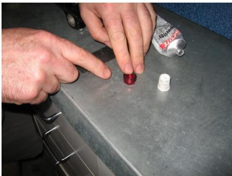
23. Prepare the 10 mm adaptor nut with RTV to help secure the
