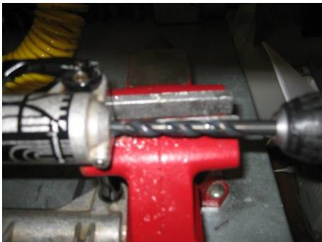
12. On the Damper leg, drill with a 10 mm drill slowly blowing off the chips to avoid falling in
