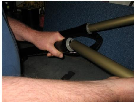
16. Grease the oil and dust seal with your choice of grease and re-assemble the slider tubes to the lower casting
