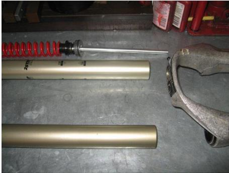
8. Remove the snap ring and rebound damper rod assembly
