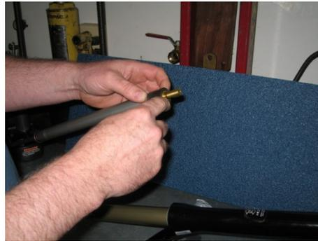
19. Apply RTV Silicone to the O-ring Groove on the bottom of the ABS Cone.
