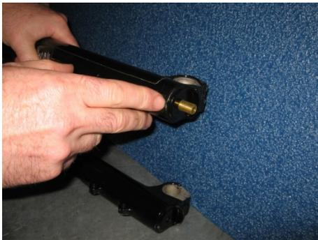
22. Push it thru until the ABS cone bottoms on the lower leg
