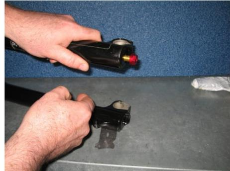
24. Thread the nut with the o-ring facing the lower leg
