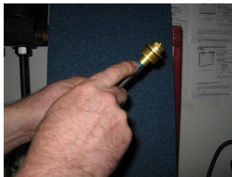
29. Screw on the fork cap. **Make sure rod bottoms out before the jam nut!**
