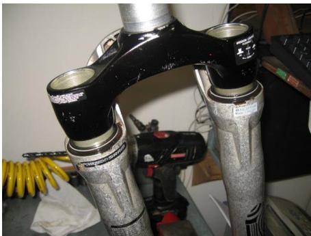
11. Bottom out against the cast lower leg. This will prevent any chips damaging the bushings and seals
