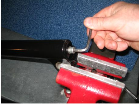
4. Using a 5 mm Allen key loosen the bolt 4-5 turns
