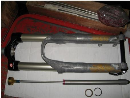
17. Prepare to install the Damping Cartridge
