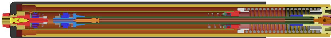
So as the air volume above the oil compresses to a smaller volume creating a much higher pressure adding a small amount of spring rate deeper in the stroke (ramp up). The damper side stanchion seals (dust wipers/seal) need to hold back this increased pressure so they must be clean and in good condition or the oil will weep out. We recommend the stock seals or SKF replacements, low friction seals will not be necessary as the seal is constantly lubricated and these seals may weep even when new.
