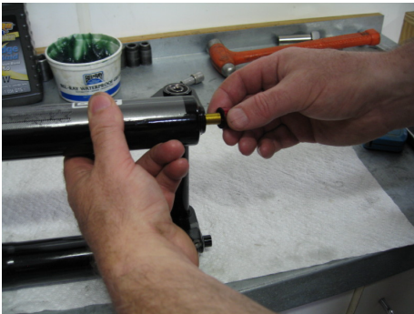
Thread the nut with the o-ring facing the lower leg shown on the Boxxer
