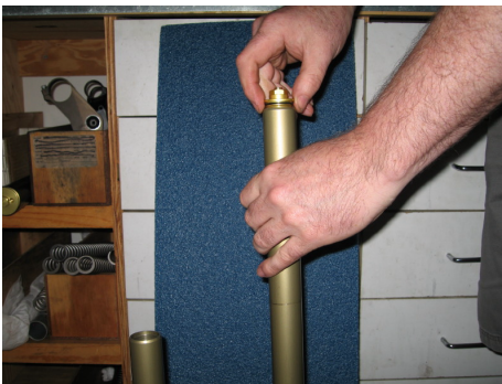
Screw on the fork cap with fork stanchion fully extended.
