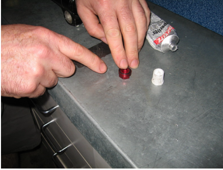
Prepare the 10 mm adaptor nut with RTV to help secure the -014 o-ring
