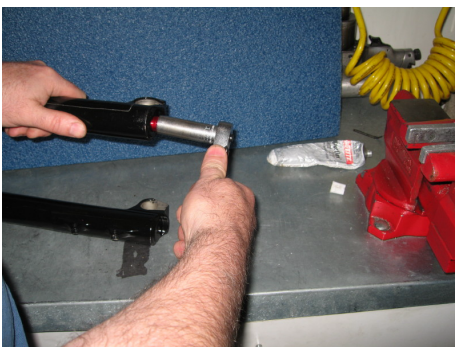
Tighten the nut to 10-15 in-lbs
