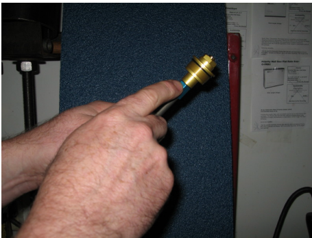
Make sure the fork cap bottoms on the cartridge rod before the jam nut
